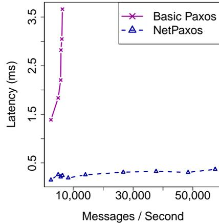
Figure 13: Evaluation of performance showing the throughput vs. latency for basic Paxos and NetPaxos.
