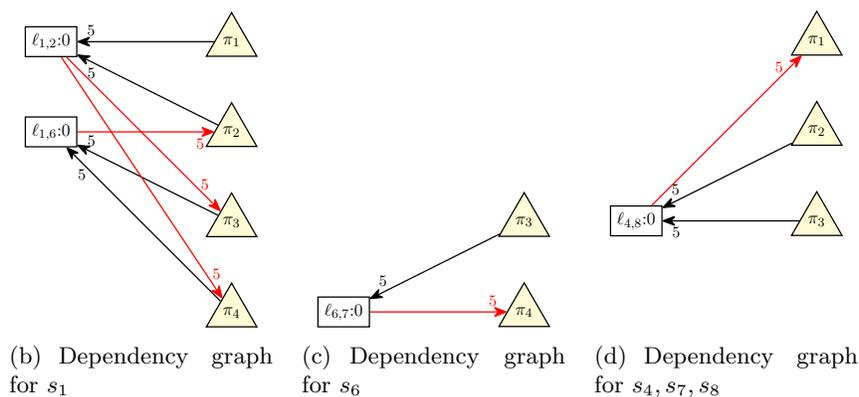
Figure 8: Decomposing a network update into three dependency graphs.
