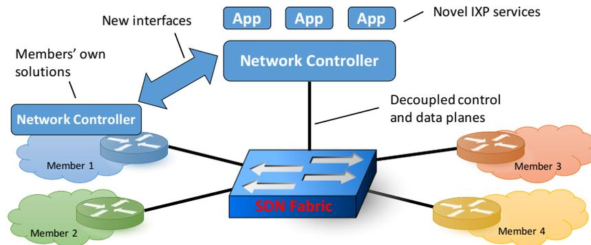
Figure 1: Preliminary architecture of an SDN-enabled IXP.
