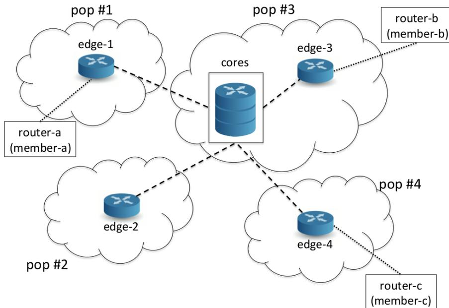
Figure 2: Typical topology of a medium to large IXP.
