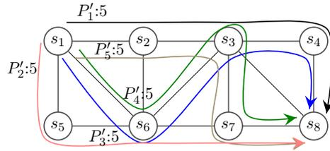
(b) Flow  $F_{1-8}$  in target configuration ( $\mathbb{C}'$ )
