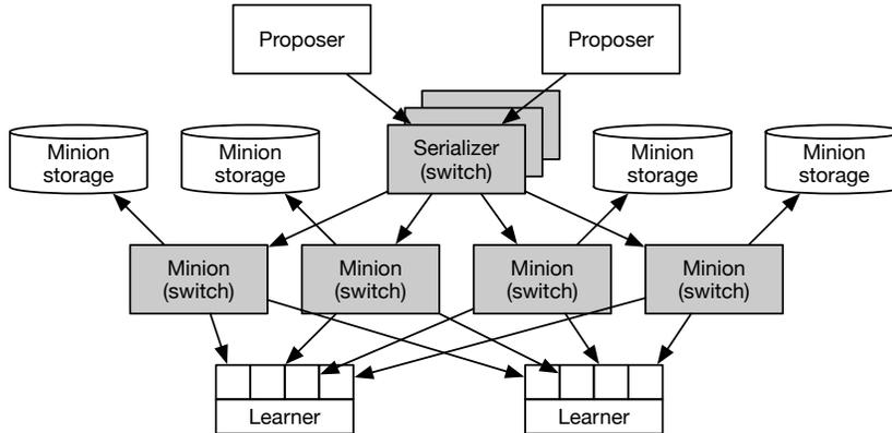
Figure 11: Network Paxos architecture. Switch hardware is shaded grey. Other devices are commodity servers. The learners each have four network interface cards.
