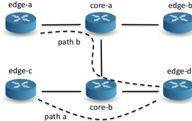
Figure 3: Example of multi-hop in the core.
